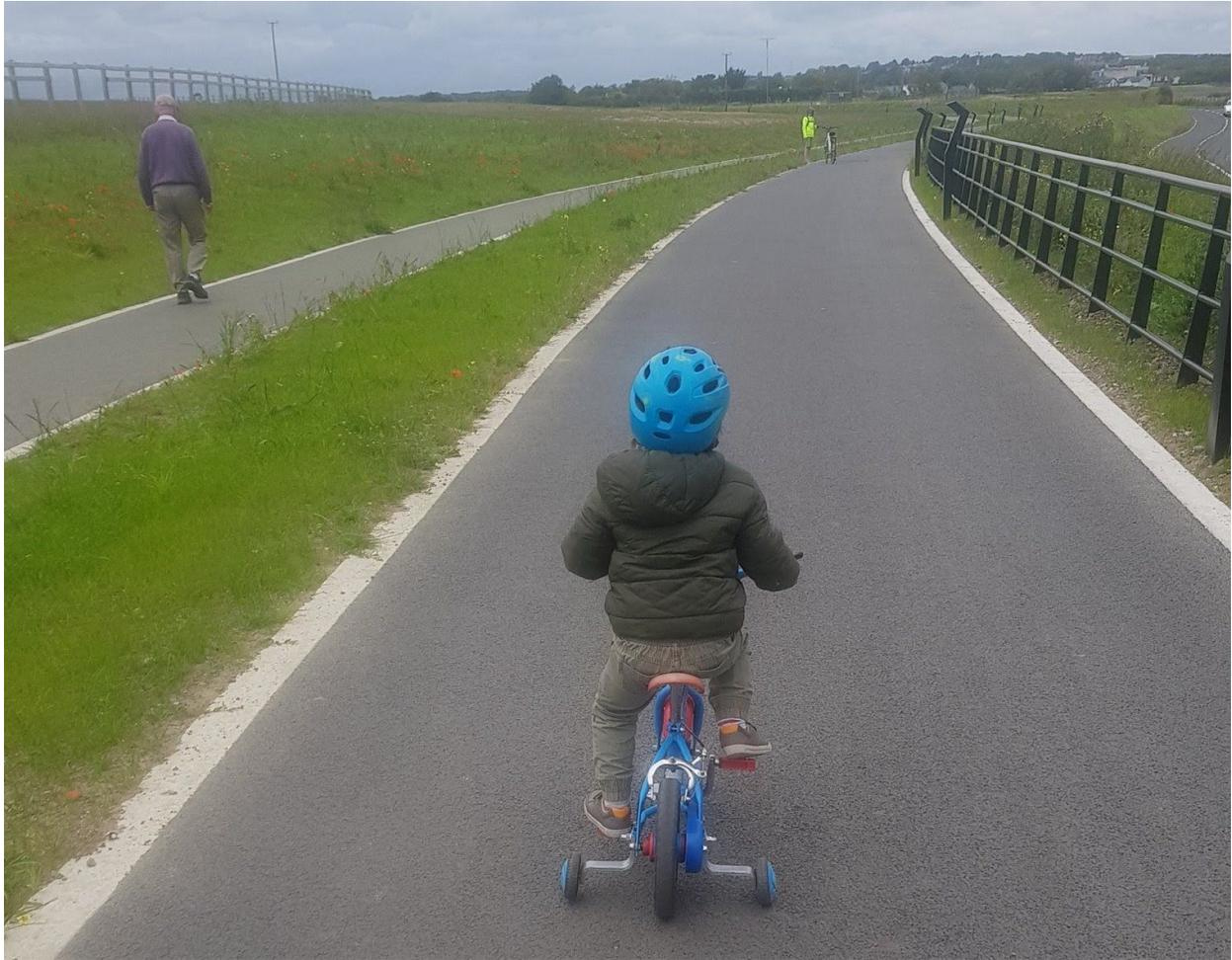
*Photo of Baldoyle to Portmarnock Greenway with a 3m cycleway, 2m footpath and grass buffer*
